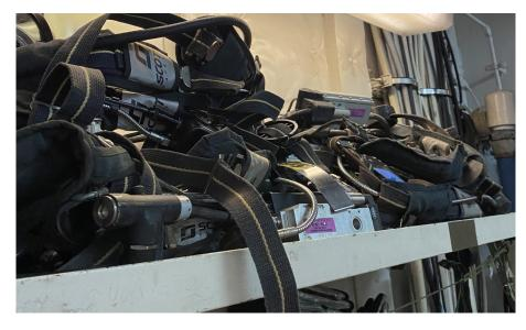
Excess firefighting equipment that is either incomplete or has overdue services. The pile of gloves is a pile of the wrong type of gloves. (Photo by: Mr. Robert Penner)
