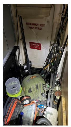
Identified emergency exit is completely blocked by excess storage, the emergency exit hatch is on the deck under everything. (Photo Credit: Mr. Robert Penner)
